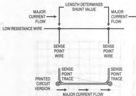
Figure 6. Detail of a Low Resistance Current Shunt
