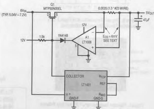
CONNECT ALL  $\oplus$  LABELED RETURNS TO A SINGLE POINT AT THE  $6V_{IN}$  SOURCE
