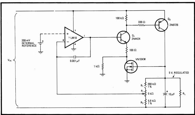
**Dropout limit.** This low-power regulator, using output transistor operating in common-emitter configuration and having large junction area, can deliver 10 mA at 5 V for an input voltage only 12 mV higher and up to 1 A at 5 V for a 6-V input. Input-to-output voltage differential is only 650 mV at load currents of 750 mA. The V-MOS field-effect transistor provides short-circuit protection in such instances.
