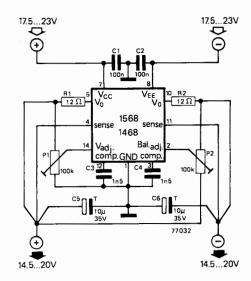
max. current 100 mA. A change in the load of 50 mA causes a variation of approx. 3 mV in the output voltage. For a current of 50 mA the minimum voltage drop across the regulator is at least 2.5 V. The noise suppression is then around 75 dB, and the stability of the output voltage is better than 1% for a variation in temperature of 75 °C. The noise at both outputs is less than 0.1 mV.
