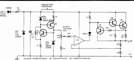
between 10 and 6 volts, so, for instance, most battery cassette equipment may be driven. Short-circuit protection is provided by Q3; when the output current exceeds 400mA sufficient voltage is dropped across R3 to turn on Q3, which shunts drive away from the base of Q4 and hence prevents the output current from rising further.
