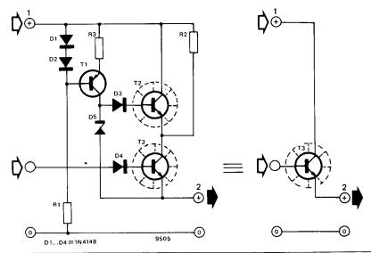
means that T2 must be cut off. The voltage at the collector of T3 is equal to the input voltage '+1' minus the voltage drop across R2. In this situation, the circuit behaves like a normal single transistor series regulator (T3) with a series resistor (R2). The maximum dissipation in T3 occurs when half the voltage difference between '+1' and '+2' is dropped across it; the load current is then:
