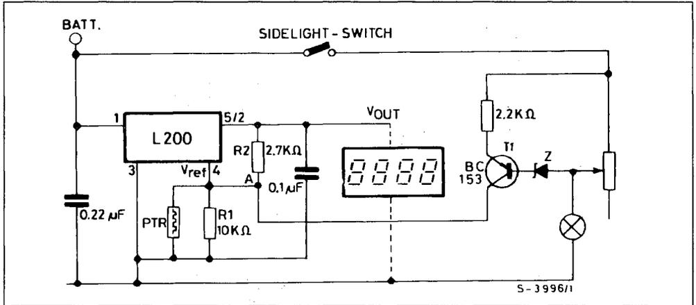
In dusk conditions, when the sidelights are switched on, T1 starts to conduct with its conduction set by the potentiometer wiper at its uppermost position the sidelights are at their brightest and current through T1 would be a minimum. With the wiper at its lowest position obviously the opposite conditions apply.
