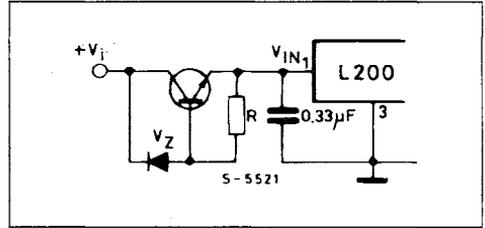
The designer must take into account the dissipated power and the SOA of the preregulation transistor. For example, using the BDX53, the maximum input voltage can reach 56 V (fig. 16). In these conditions we have 20 V of  $V_{CE0}$  on the transistor and with a load current of 2 A the operation point remains inside the SOA. The preregulation used in fig. 16 reduces the ripple at the input of the device, making it possible to obtain an output voltage with negligible ripple.
