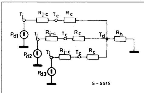
This applies if the various dissipating elements are fairly near to one another with respect to the heat-sink dimensions, otherwise the heatsink can no longer be considered as a concentrated constant and the calculation becomes difficult.
