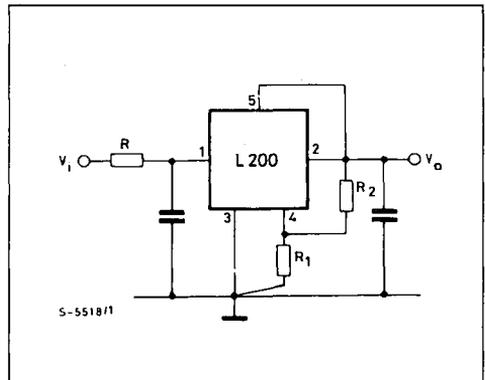
Where  $V_{drop}$  is the minimum differential voltage between the input and the output of the device at current  $I_O$ .  $V_{i \min}$  is the minimum voltage.  $V_O$  is the output voltage and  $I_O$  the output current.
