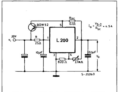
The latter is given by :  $I_{REG} = I_B + \frac{V_{BE}}{R}$
