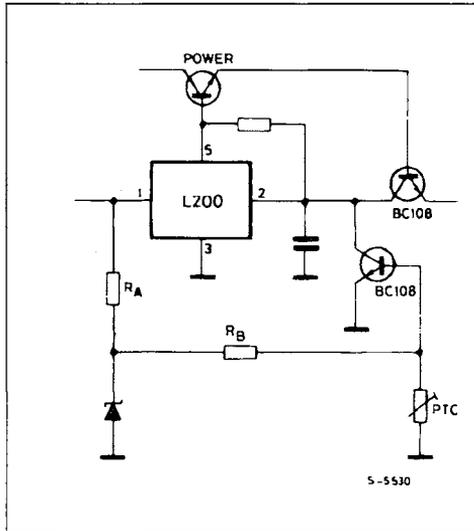
VOLTAGE REGULATOR FROM 0 V TO 16 V - 4.5 A
