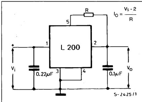
The output current  $I_o$  is fixed by means of R :
