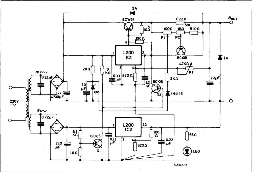
POWER SUPPLY WITH  $V_o = 2.8$  TO  $18$  V,  $I_o = 0$  TO  $2.5$  A
