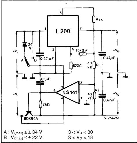
Since the maximum supply voltage of the op amp used is  $\pm 22 \text{ V}$ , when pin 7 is connected to point B output voltages up to about  $18 \text{ V}$  can be obtained. If on the other hand pin 7 is connected to point A, much higher output voltages, up to about  $30 \text{ V}$ , be obtained since in this case the input voltage can rise to  $34 \text{ V}$ .
