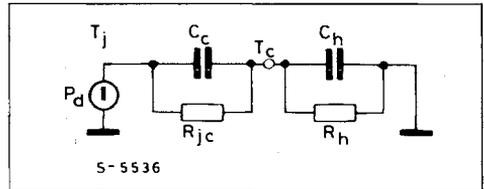
Where  $C_c$  is the thermal capacitance of the die plus that of the tab.
