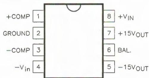
Figure 8. RC4195 pinout.
