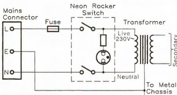
Figure 14. Mains wiring.
