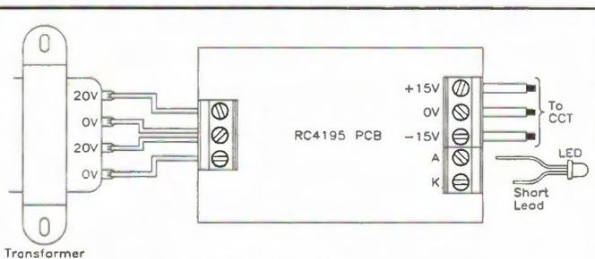
Figure 13. Transformer/PCB wiring.
