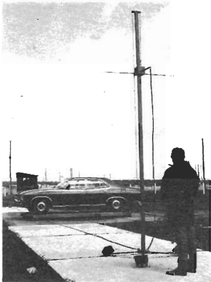
Fig. 5. Measurement of ignition interference.
