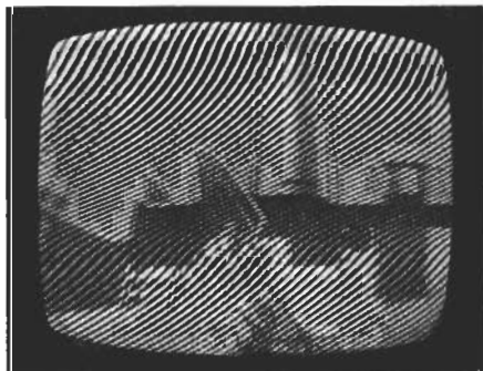
Harmonic interference. This appears as a series of lines, or a herringbone pattern, on one or two channels at once. The source is often a nearby transmitter
