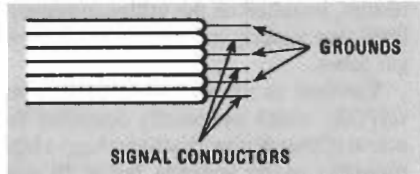
FIG. 3—TO ELIMINATE CROSSTALK problems in ribbon cable, alternate conductors should be grounded.
