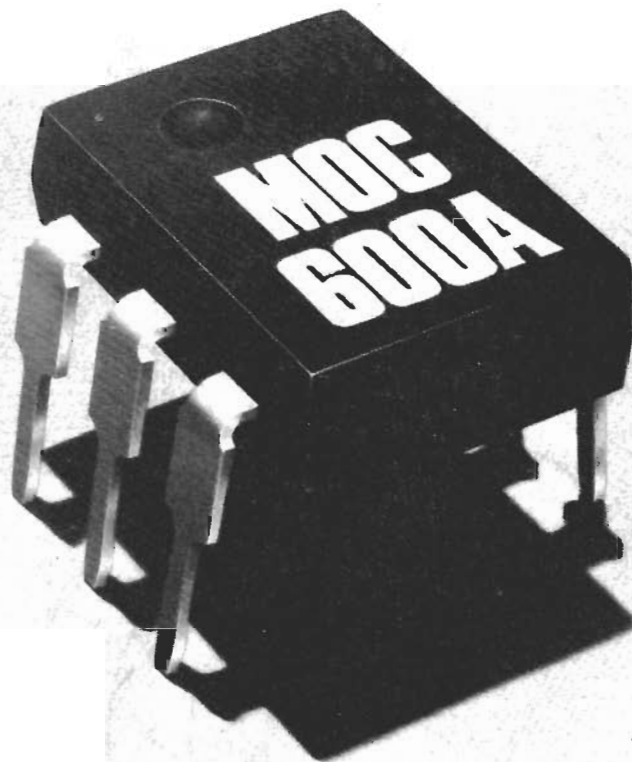
OPTO-ISOLATORS, such as the members of the Motorola MOC600A family, are inexpensive and readily available.
