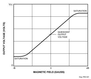
Figure 1: Linear Hall Sensor Transfer Curve
