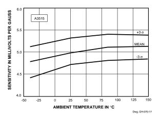
Figure 17: Sensitivity vs Temperature (A3515)
