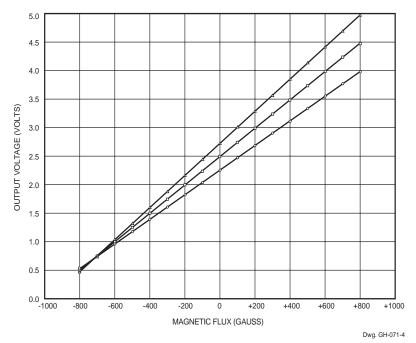
Figure 4: Linear, Ratiometric Hall-Effect Sensor Characteristics (A3516 Output) Table 3: Linear, Ratiometric Hall-Effect Sensor Measurement Data (A3516)
