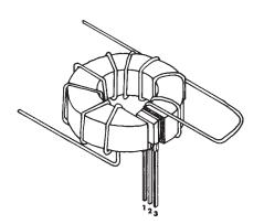
Figure 6A: Toroidal Current Sensor (<15 A)
