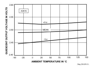
Figure 13:  $V_{OQ}$  vs Temperature (A3515)
