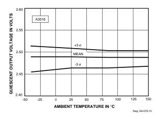
Figure 15:  $V_{OQ}$  vs Temperature (A3516)
