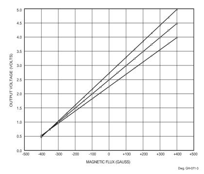
Figure 3: Linear, Ratiometric Hall-Effect Sensor Characteristics (A3515 Output) Table 2: Linear, Ratiometric Hall-Effect Sensor Characteristics Measurement Data (A3515)
