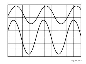
Figure 8: V<sub>OUT</sub> (Upper) vs I<sub>IN</sub> (Lower) at 10 kHz
