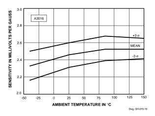
Figure 19: Sensitivity vs Temperature (A3516)
