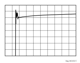
Figure 11: A3506 Power-Up (2.0 μs/Div.)
