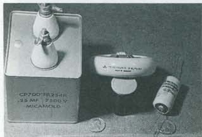
FIG. 9—HIGH-VOLTAGE CAPACITORS. A 0.25 \mu F, 7.5-kilovolt capacitor is on the left; a 100 pF, 15-kilovolt capacitor is in the middle; and 0.0005 \mu F, 5-kilovolt capacitor is on the right.
