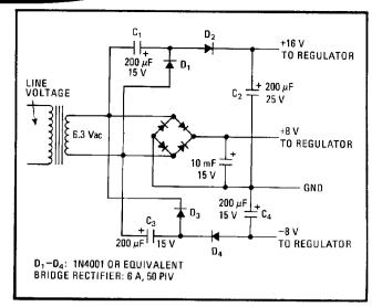
**Add-on sources.** Voltage-doubler circuits, added to full-wave bridge rectifier, provide extra positive and negative voltage supplies. Bridge provides over 2.5 A at +8 V to drive a regulator IC for +5-V output. Upper doubler delivers 50 mA at +16 V for regulation to +12 V, and lower doubler delivers 50 mA at -8 V for regulation to -5 V. The extra sources meet the voltage and current requirements of microprocessor peripherals that cannot use the +5-V source.
