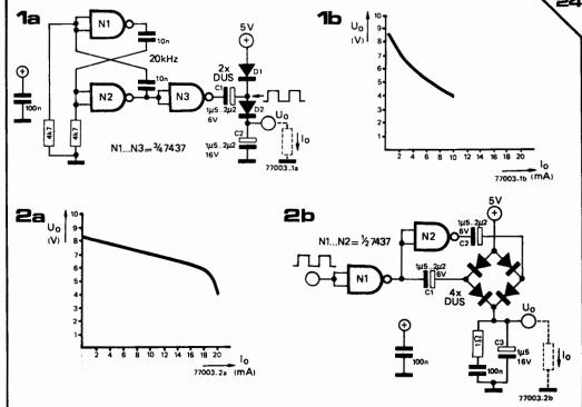
that have only a 5 V supply rail, where a higher voltage is required at a low current. Figure 1a shows the basic circuit, which uses three of the gates in a 7437 quad two-input NAND buffer IC. N1 and N2 are connected as a 20 kHz astable multivibrator, and the output of N2 drives N3, which acts as a buffer between the astable and the doubler circuit. When the output of N3 is low C1 charges through D1 and N3 to about +4.4 V.
