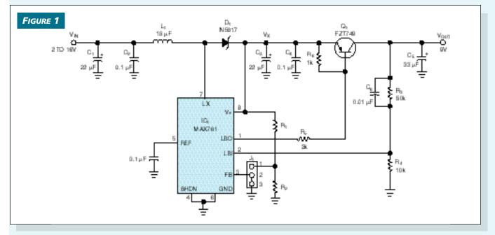
Toggling between switching and linear operation, this regulator operates with input voltages above and below the desired output voltage.
