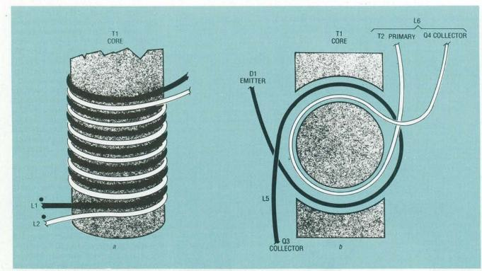
FIG. 6—TRANSFORMER T1 IS MADE by winding coils L1 and L2 first (a). After putting a layer of cellophane tape on top of the first windings, coils L3 and L4 are wound on top of L1 and L2. Coils L5 and L6 are wound after the transformer is mounted on the board (b). See text for detailed instructions.
