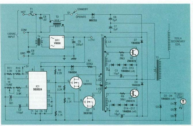
FIG. 2—SCHEMATIC FOR THE SOLID-STATE TESLA COIL. The secondary of the Tesla coil appears like a series RLC circuit due to the self-capacitance of the coil with respect to ground.
