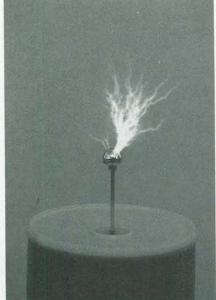
FIG. 7—SEEN HERE IS THE DISCHARGE from the ball electrode into the air.
