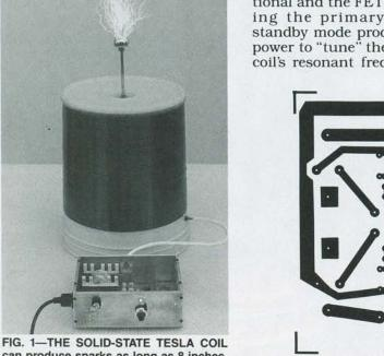
can produce sparks as long as 8 inches. The output reaches a peak of about 100,000 volts.
