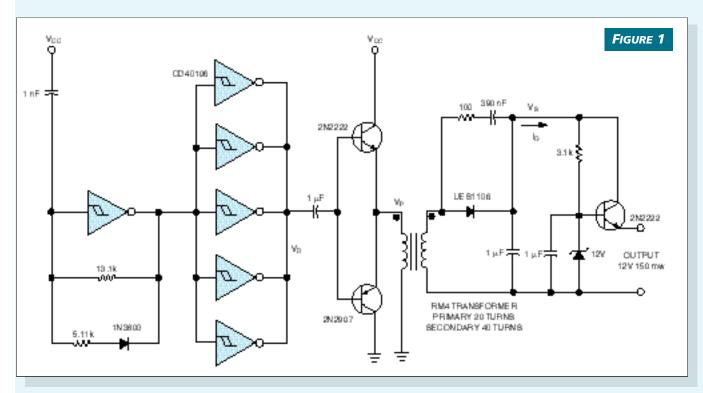
A simple CMOS oscillator, an inexpensive transformer, and a few components form a low-cost, galvanically isolated dc/dc converter
