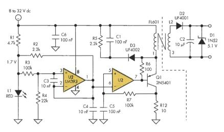
Dual comparators act as a low-cost dc-dc converter with a simple common-mode choke serving as the isolation transformer.
