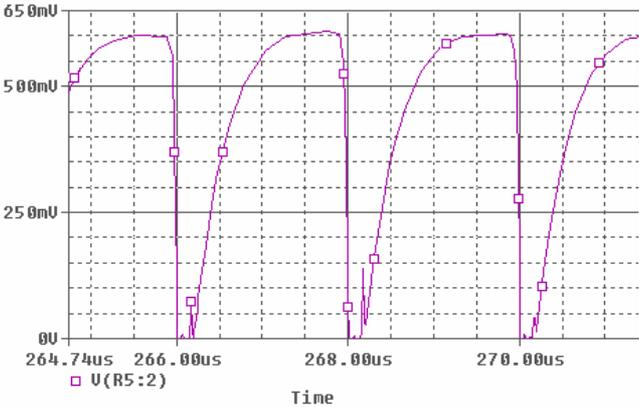
Figure 26 – Current sense signal
