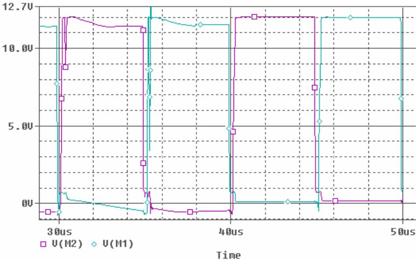
Figure 12 – Gate driver pulses
