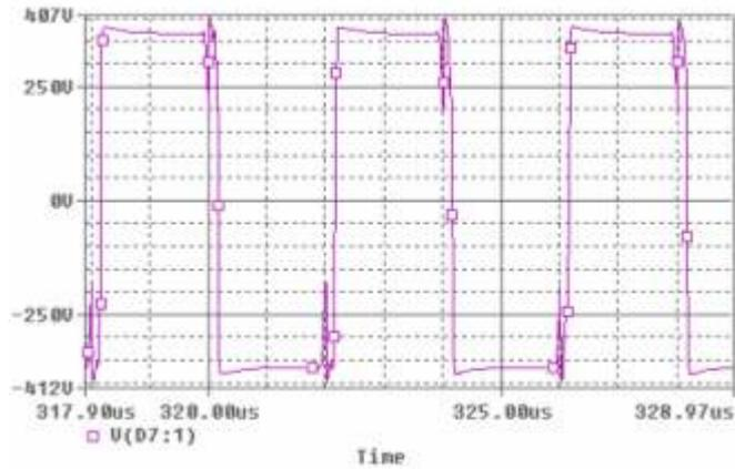
Figure 28 – Secondary output before rectification
