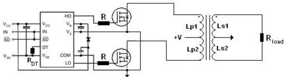
Figure 10 – Test Bench for transformer testing
