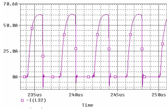
Figure 31 – MOSFET drain current
