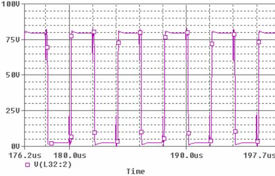
Figure 27 – MOSFET drain voltage
