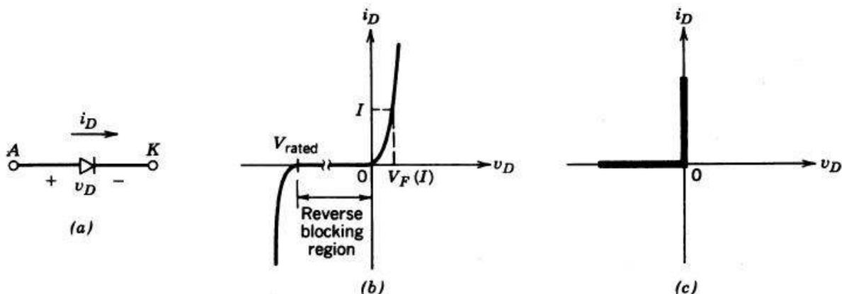
Figure 4 – Diode characteristics
