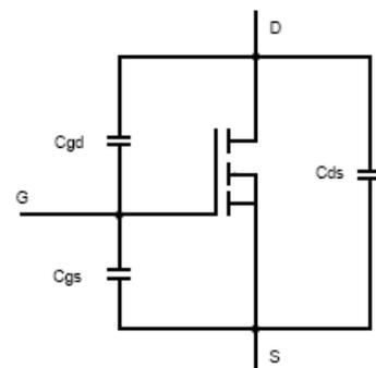
Figure 6 – Internal capacitances
