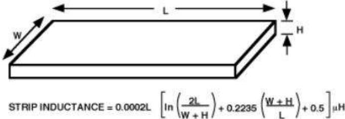
Figure 9 – Calculating strip inductance
