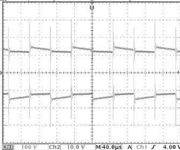
Figure 15 - Output before rectification
