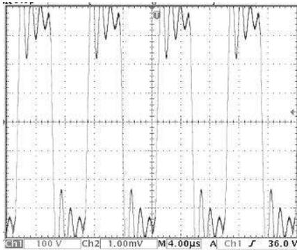
Figure 20 –  $V_{sec}$  before rectification
