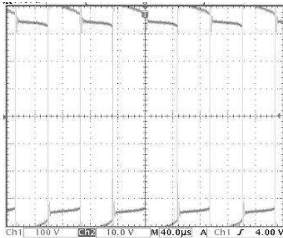
Figure 17 – Output before rectification
