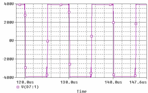
Figure 21 –  $V_{sec}$  before rectification
