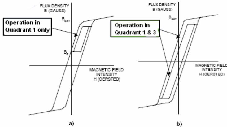
Figure 1 – Uni-Directional and Bi-Directional flux swing
