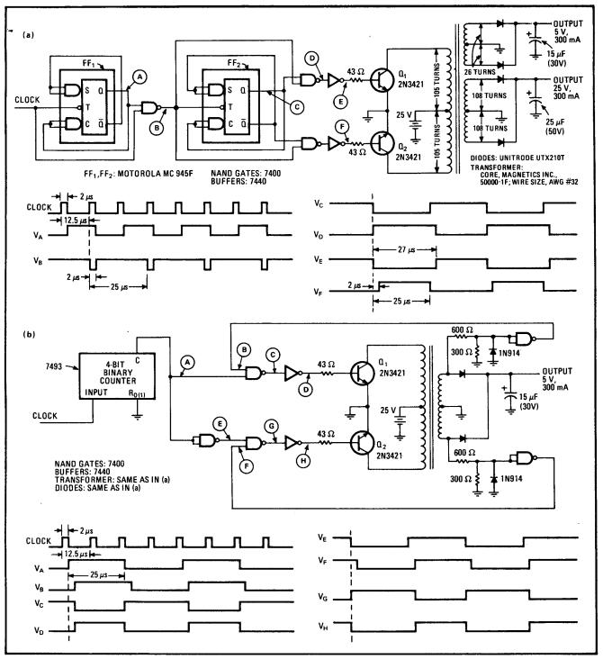
**Improving dc-dc converter efficiency.** These dc-dc converters employ push-pull inverter transistors that switch at 20 kilohertz. Conventional digital ICs are used to delay the drive signals to the switching transistors so that these devices cannot conduct simultaneously, causing unwanted current spikes. The converter in (a) has a fixed delay, while the delay of the converter in (b) depends on a feedback signal voltage.
