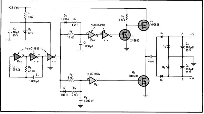
**Converter.** Unlike standard dc-dc converters, this circuit gives two dc voltages, one of positive, one of negative polarity—without using transformers or inductors. Only one inverter chip, three transistors, and a few discrete components are needed to realize the converter. Diodes  $D_5$  and  $D_6$  determine the level of positive and negative voltages at terminals A and B.
