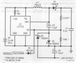
Figure 2. DC to DC Converter Generates –24V from 3V or 5V
