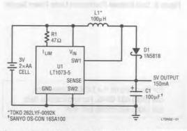
Figure 1. Two "AA" Cell to 5V Step-Up Converter Delivers 150mA
