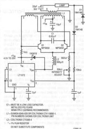
Figure 3. Cold Cathode Fluorescent Lamp Power Supply
