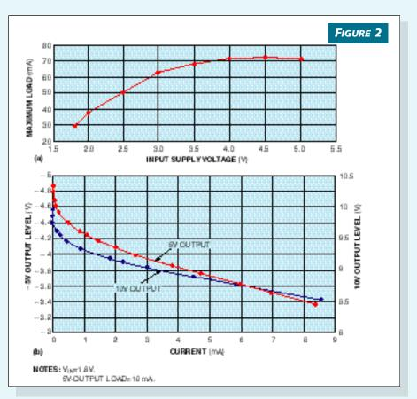
With auxiliary rails unloaded, the 5V output's maximum available load current rises with input supply voltage (a). The auxiliary-output voltage levels depend on the load current (b).
