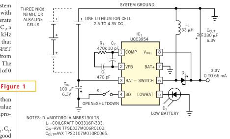
This 3.3V dc/dc converter takes full advantage of the benefits of an Li-ion battery and works over the battery's full range of 4.2 to 2.5V.
