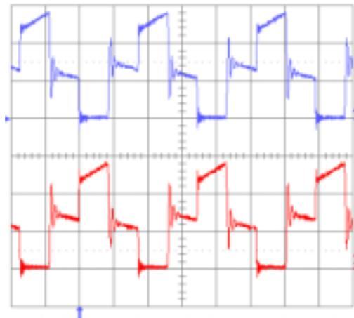
( Current waveform on the secondary windings)
