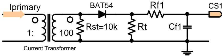
**Current transformer: Pulse P8208 Turns ratio:**  $CT_{tr} := 100$
