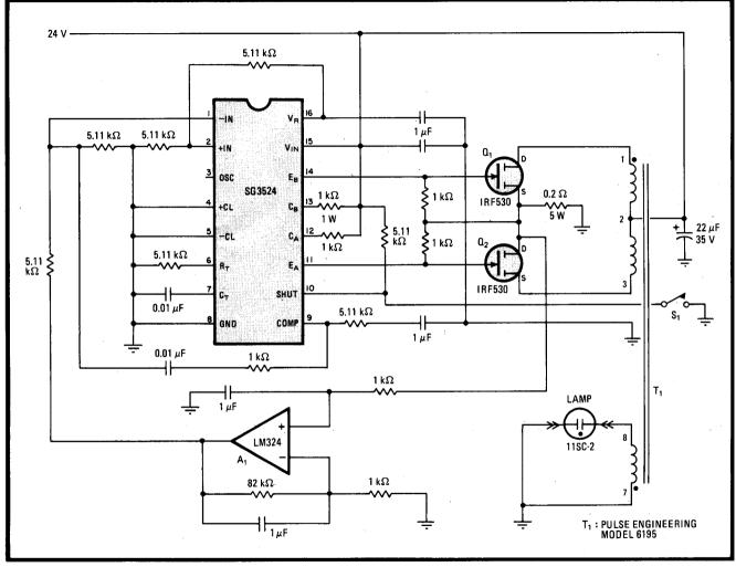
**Arc-over.** Low-power transistor-driven inverter generates high-voltage square wave to fire fluorescent and mercury-vapor lamps and provides low current to maintain ionization. Symmetry of inverter's output prohibits build-up of ions at lamp's cathode, thus increasing operating life.
