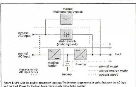
and the load. Power for the load flows continuously through the inverter.
