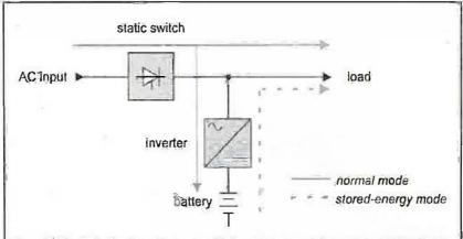
Figure 4. UPS with the line-interactive topology, The inverter is connected in parallel and acts to backup utility power. It also charges the battery. Through its reversible operation, it interacts with utility power.
