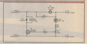
relay contacts close, giving full charge to the battery. RV1 is adjusted to give the correct change-over voltage.
