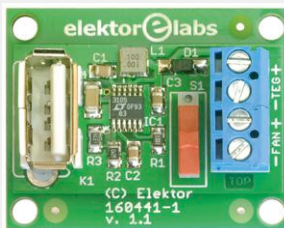
Figure 5. The assembled converter board.
