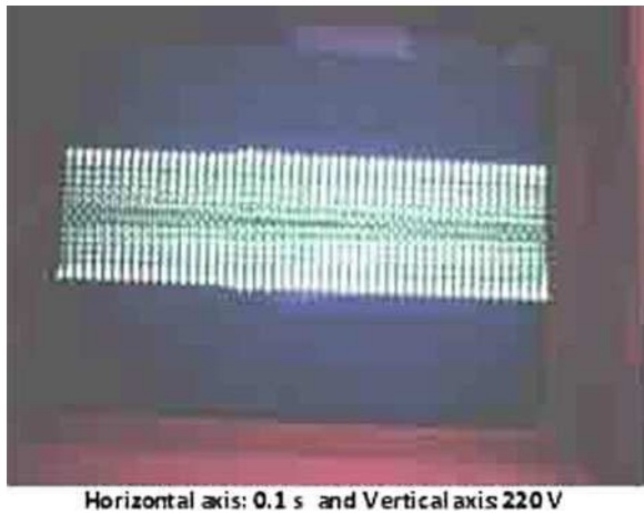
Fig. 6.31 Tap-changer output voltage waveform in no-load case for quick rise of input voltage from 175 V to 240 V
