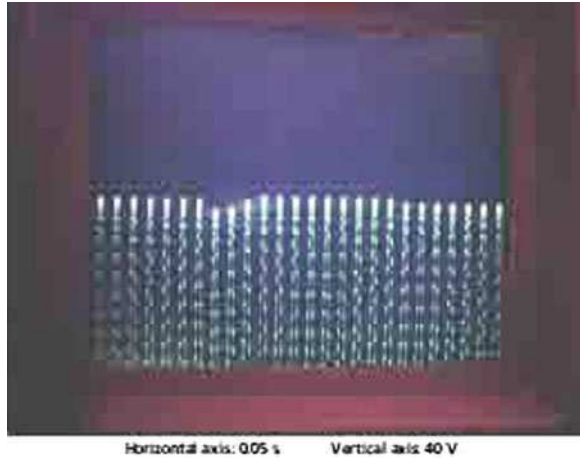
Fig. 6.41 Tap-changer output voltage for change of load current from 0 to 5 A at input voltage 224 V
