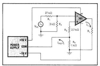
**Uncritical.** Load current produced by this circuit depends on input voltage, not load resistance. Circuit does not require matched resistors for accurate control of current, but power supply must float.
