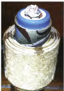
Part of disassembled 18650 Li-ion cell, with a section of the "Swiss Roll" cut away to show the inside construction.
