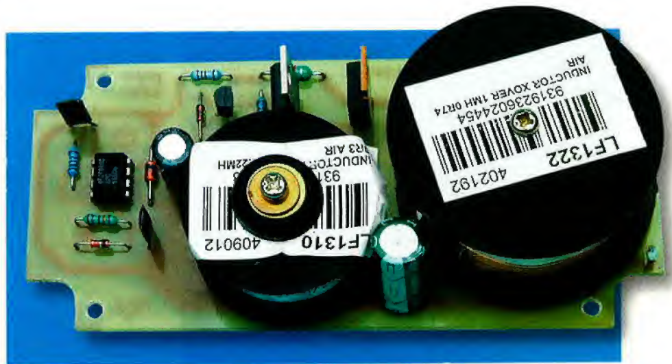
The large inductors on this prototype unit were secured using spacers, screws and washers but the final version uses cable ties to secure the inductors instead.
