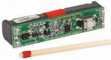
Figure 5 Reference designs can provide low-risk platforms for developers to more quickly understand how to use a boosted single battery in their designs.
