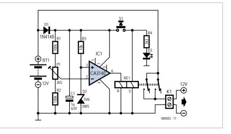
the battery voltage rises above the reference voltage again, the reset coil will no longer be powered and the current consumption drops back to about 2.5 mA.
