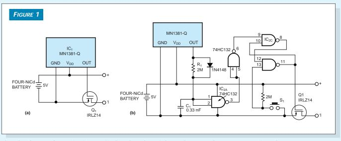
These low-battery-detect circuits cut off when the voltage is lower than 4V and consume approximately 1.2 mA.
