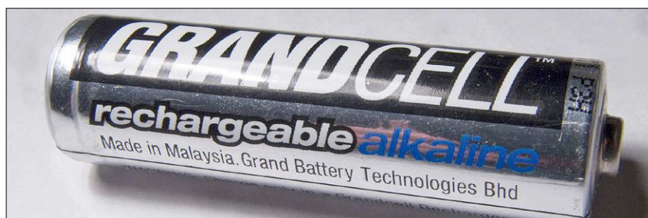
Figure 7. RAM battery cell based on an alkaline manganese chemistry in a standard AA package. These batteries must not be subjected to deep discharge and require a special charger.
