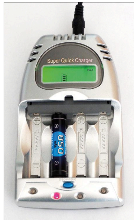
Figure 11. Intelligent quick-charger for four AA- or AAA-size NiCd or NiMH cells working at up to 0.8C. The device can even detect defective batteries. A press of the blue button discharges the cells before the charging cycle starts
