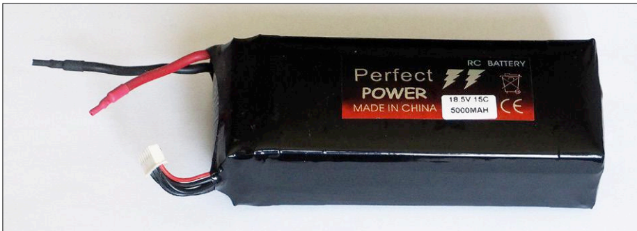
Figure 4. Type 5s1p Lithium polymer battery rated at 18.5 V and 5 Ah. The maximum discharge current is 15 C, or 75 A, and the pack is designed for use in radio-controlled models. The small six-way connector allows a charge balancer to be connected.
