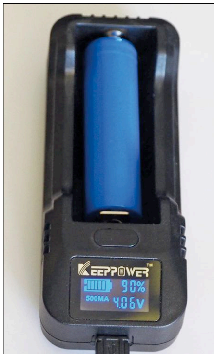
Figure 10. Low-cost charger for 18650-size LiCoO 2 cells with a USB connection and OLED display.
