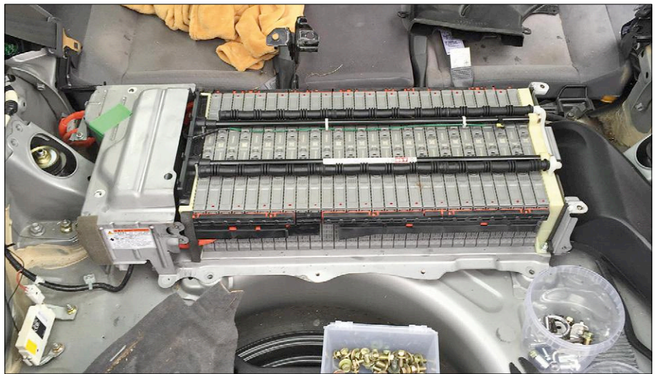
Figure 2. Inside the battery of my old Prius II hybrid vehicle: 28 modules each comprising six Panasonic prismatic NiCd cells rated at 1.2 V and 6.5 Ah wired in series, giving a total of 201.6 V. The pack can store 1.3 kWh and weighs in at 39 kg.
