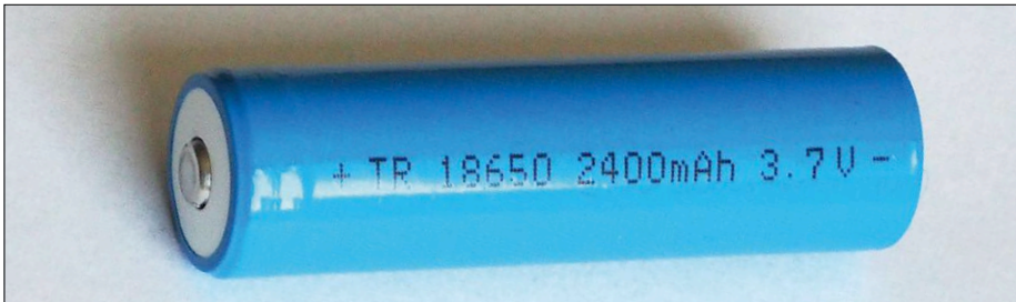
Figure 5. This typical lithium battery in 18650 format is based on an \text{LiCoO}_2 chemistry. Such cells are becoming more popular in flashlights and especially in solar garden lights. The nominal voltage is given as 3.7 V rather than 3.6 V.
