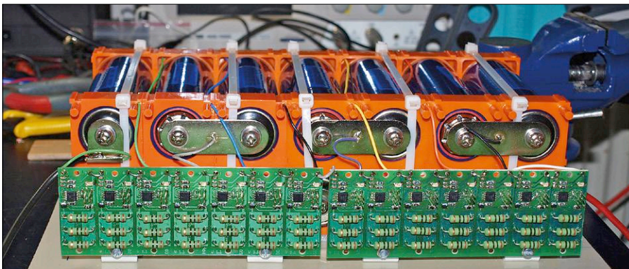
Figure 6. The 45-V \text{LiFePO}_4 pack from my Segway clone: 14 type 38120 cells rated at 9 Ah and 10C. In the foreground is the charge balancer.
