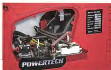
The modified control panel of the Powertech (Jaycar) 1kW Generator. At left is the two-pin microphone socket we added (about the only spot possible!). Centre is a close-up of the wiring and right is the panel about to go back in.
