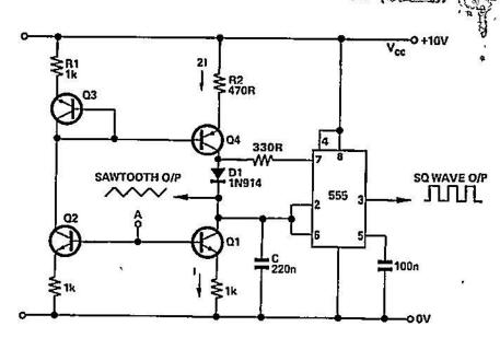
cycle recommences; the repetition frequency is determined by the magnitude of I, which is set by the voltage applied at the input point A.
