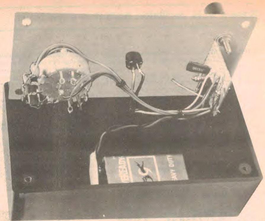
This view inside the case shows the general layout of the oscillator. The stripboard assembly is soldered directly to the black terminal post tag, as shown on the component overlay diagram.
