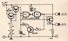
This sawtooth waveform generator which is built round a current controlled oscillator is distinguished by its large sweep range. It is suitable for use in electronic music applications, and the narrow output pulse also enables the circuit to be used as a pulse-CCO for sample/hold circuits.
