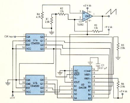
To ensure that the rail-to-rail ramp goes from 0 to 5 V, the negative voltage driving the DAC08 must be greater than -8.5 V.
