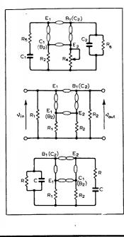
Typical data  $Tr_1 BC126$ ,  $Tr_2 BC125$   $R_1$ ,  $R_2 10k\Omega$ ,  $R_3 5k\Omega$   $R_4 4.66k\Omega$   $R_5$ ,  $R_6 4.7k\Omega$   $C_1$ ,  $C_2 0.1\mu$ F  $V_s \pm 5V$ Ratio required of  $R_2$ :  $R_4$  slightly greater than two to allow for component tolerances Frequency 373Hz (maximum 20kHz)  $v_{out}$  1.55V pk-pk, 0.3V offset
