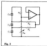
progressively less attenuated. When oscillations are vigorous, and distortion ensues, these harmonics are fed back introducing intermodulation distortion and shifting the frequency of oscillation away from the 180° phase-shift frequency of the network.
