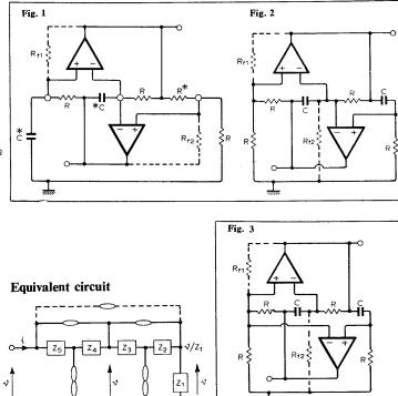
produce sustained oscillation. For  $Z_1 = Z_2 = Z_3 = Z_5 = R$  and  $Z_2 = 1/j\omega C$ ,  $Z_1 = j\omega C R^2$ .
