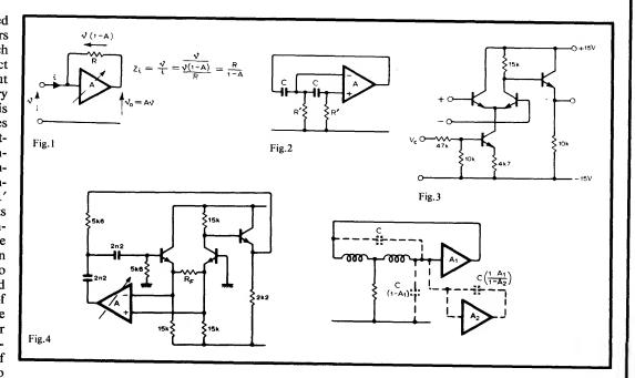
effect can be applied to LC oscillators to replace a capacitor that normally appears in a feedback path by either a grounded capacitor or one connected across a separate amplifier. If  $A_1$  is fixed to sustain oscillations, then  $A_2$  varies the effective capacitance and hence the frequency without disturbing the amplitude condition.
