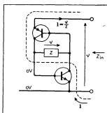
zero giving  $C_1/C_2 + R_2/R_1 = 1$ or  $R_1 = 2R_2$ ,  $C_1 = C_2/2$  and  $f=1/2\pi\sqrt{C_1R_1C_2R_2}.$
