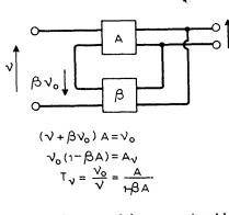
Fig. 1. A fraction of the output is added to the source at the input in deriving a standard form of the basic feedback equation. Positive feedback occurs when  $\beta A$  is positive.
