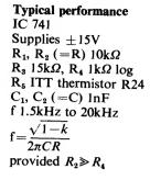
but the need for a twin-gang control which normally requires a good match is avoided. A further advantage of this circuit is that low frequencies are obtained without using large values of capacitance. Provided the thermistor has a long enough thermal time constant, frequencies down to 10Hz are possible with capacitances of  $0.1\mu F.$
