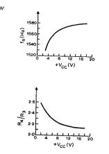
Typical performance +V<sub>cc</sub>+10V, 2mA  $R_1$ ,  $R_2$ , R 10k $\Omega$ , C 10nF  $R_3+R_4$  10k $\Omega$  (realized with 10k $\Omega$  potentiometer to adjust loop gain)  $Tr_1$ ,  $Tr_2$  1/5×CA3086 (Note  $Tr_1$  or  $Tr_2$  emitter is pin 13)
