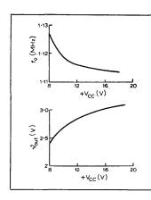
output waveform. The more the gain exceeds the critical value the more distorted will the output waveform become and the lower will be the frequency of oscillation. (See graphs for effect of increasing supply voltage, for example, after setting the critical condition at a lower value of +Vcc.)
