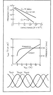
t.h.d. 1.2%. For 470k $\Omega$ , V<sub>out</sub> 4.4V pk-pk, t.h.d. 0.3%. R<sub>2</sub> 7.8M $\Omega$  V<sub>out</sub> 6.8V pk-pk, t.h.d. 0.6%. For 4.7M $\Omega$ , V<sub>out</sub> 4:1V pk-pk, t.h.d. 0.2%. For all above alterations, frequency does not change more than 0.2%. Variation with supply C<sub>1</sub>, C<sub>2</sub> shown on graphs.
