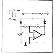
sinusoidal negative feedback and limited positive feedback can be obtained as shown above. It can be shown<sup>1</sup> that for this circuit the output is given by  $2qE\sqrt{2}/\pi$  volts r.m.s. A possible voltage-controlled limiter is shown above
