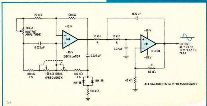
synchronous motor over a range of 48 to 74 Hz. It is used to adjust the tape speed of a recorder in the lab to that of an airplane's recorder so that the data can be recovered from airborne equipment that lacks a frequency-regulated power source.
