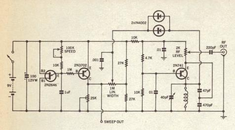
This tends to counteract the non-linear capacitance voltage characteristic of the diodes.
