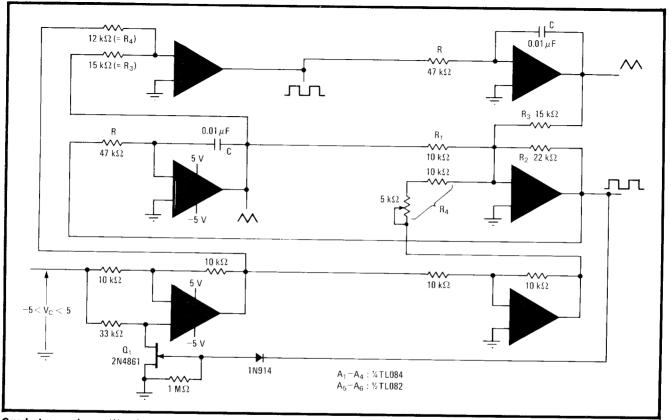
**Quadrature variance.** Waveform generator that normally produces in-quadrature (90° departure) triangular or square waves is converted into variable phase-delay circuit when gain-switching amps  $A_5$ – $A_6$  are added.  $A_5$ – $A_6$  act to advance  $A_3$ 's turn-on transition, so that signals at  $A_3$  and  $A_4$  lead those at  $A_1$  and  $A_2$ . Phase shift between both sets of waves is controlled by  $V_C$ .
