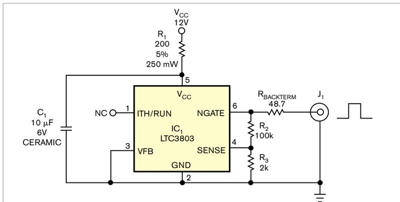
Figure 1 Switching-regulator-controller IC<sub>1</sub> delivers pulses with 1.5-nsec rise and fall times into a 50Ω load.
