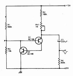
This simple pulse generator produces 100 nanosecond negative pulses of 8 volts amplitude.
