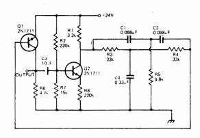
The frequency of oscillation of this circuit is determined by a twin T network and is stable to within 0.05% for  $\pm$  10% supply variation.
