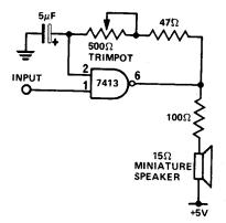
For monitoring slow logic pulses a Schmitt trigger is connected as an oscillator. The trimpot controls the pitch of the output. Very useful as a keying monitor or digital clock alarm. When the input goes high, the 7413 will oscillate.
