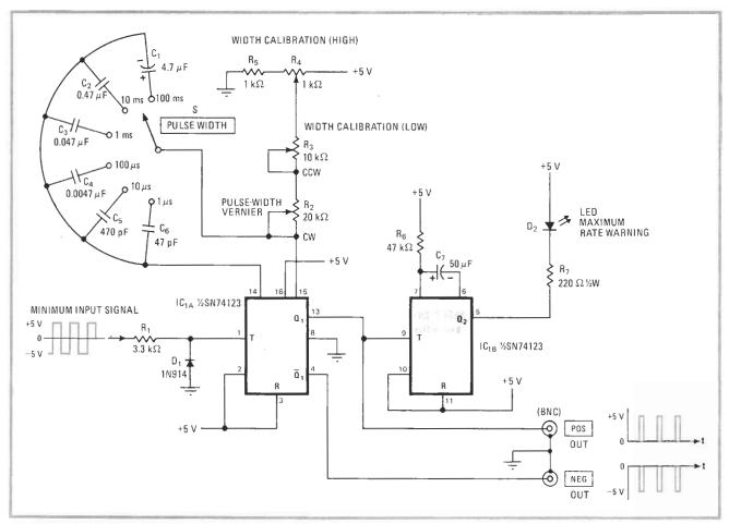
Fast and narrow. Adjustable-width pulses down to 100 nanoseconds are produced at rates to 10 megahertz by this TTL circuit, based on a single dual-monostable integrated circuit driven by any suitable clock. If the input clock rate is raised so high (or the output pulse width is made so small) that the width exceeds the period, Q<sub>2</sub> goes low and lights the warning LED.
