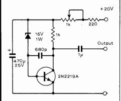
justable to zero by the potentiometer. Without the 680pF capacitor the noise extends up to 30MHz with a wideband level of more than 5V.
